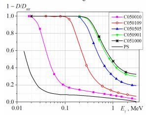
Fig. 3. The weakening of the absorbed dose of gamma radiation with a protective layer of the composite material.
