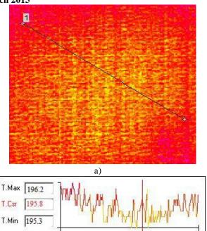
Fig. 2. Thermo gram of temperatures on surface of the mixture (a). Graph of change of temperatures on surface of the mixture (b). Melting polystyrene.
