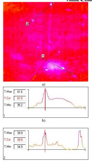
Fig. 1. The thermo gram surface temperature of the mixture (a). The graphs of temperature change along the sections 1, 2 (b, c). Beginning of the manufacturing process.
